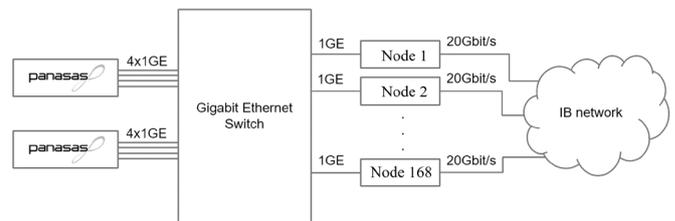
Fig. 4. Scheme of connecting Panasas ActiveStor 8 to the supercomputer SKIF Ural
