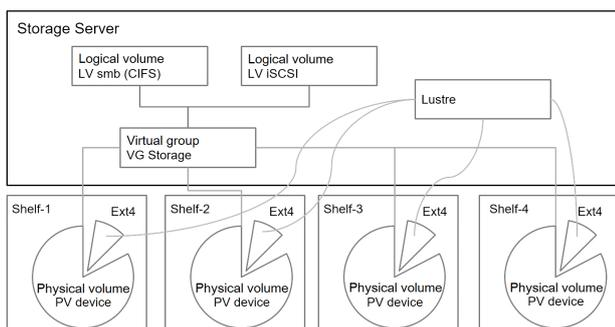
Fig. 3. Logical scheme of connecting AXUS storage system to supercomputer Tornado SUSU
