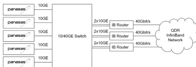
Fig. 2. Scheme of connecting Panasas ActiveStor 11 to the "Tornado SUSU" supercomputer network
